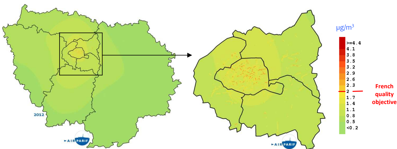
Figure 29: benzene annual mean concentration in the Paris region, background and roadside, focus on Paris and near suburbs, 2012
